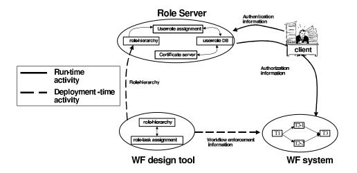
Figure 2: Security Architecture for Secure Workflow (WF) System: User-Pull Style
